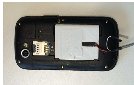
Fig. 2. 3D printed dummy battery fixture placed in the mobile phone battery slot with the power cable connected to the DC power supply output interface.
